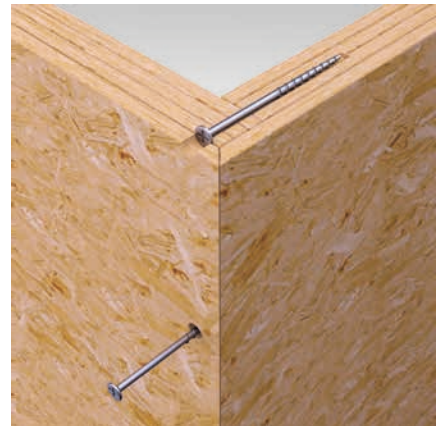
90° inside wall corner
